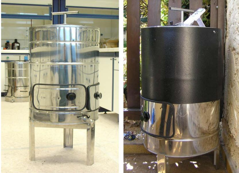
Fig. 1. The prototype household composting system.
